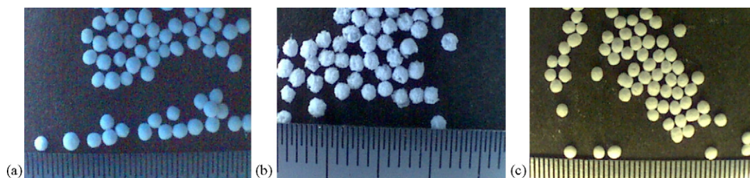
Fig. 1. Granules obtained from the spheronisation of MCC/PG paste extruded at 625 \text{ mm s}^{-1} through a 1 mm diameter die of length 4 mm: (a) wet; (b) oven-dried; (c) freeze-dried granules. The scale shows 0.5 mm divisions.
